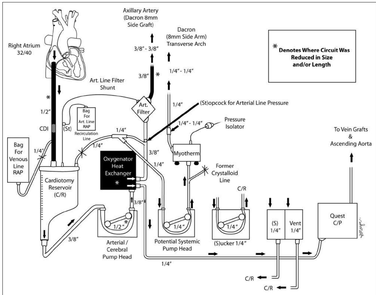
**Figure 2.** Schematic of CPB Circuit.
